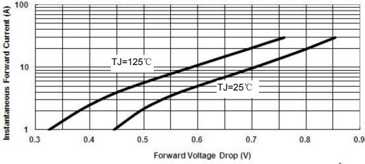
Fig.3-Typical Instantaneous Forward Voltage Characteristics
